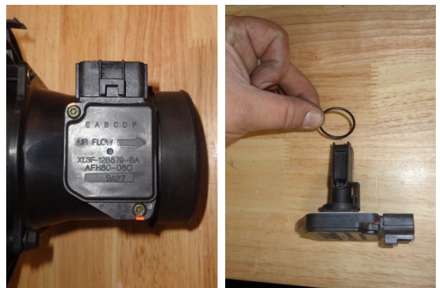
18. Remove the MAF sensor from the duct (TR20 tamper-resistant Torx bit required), then remove the sensor's o-ring.
