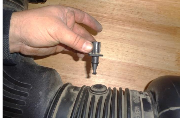
16. Firmly grasp and twist the air inlet temp sensor, and pull it from the inlet duct.
