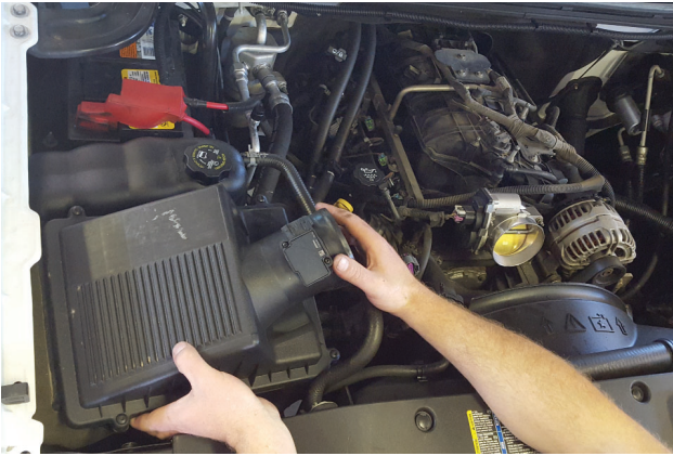
6. Lift up to release push-in grommets and remove airbox from vehicle.
