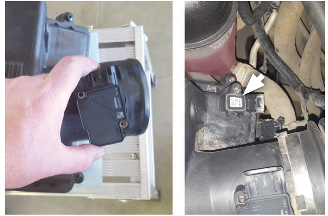
9. Remove and retain MAF sensor from factory air box. If applicable, remove MAP sensor from air box beside MAF sensor where shown.
