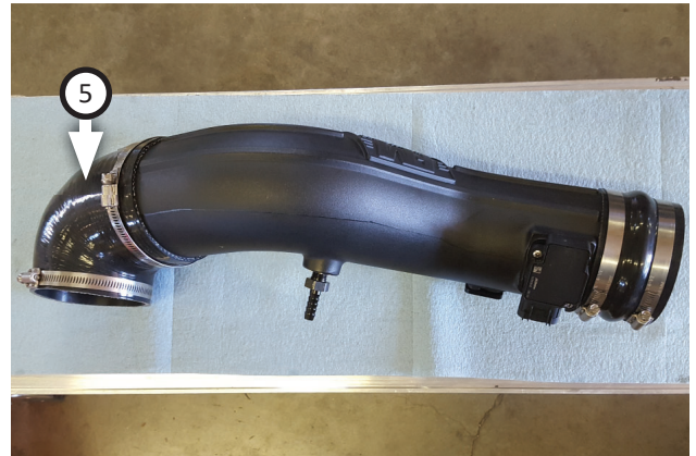
16. Place (x2) hose clamps (7) onto both sides of coupler (5) , then fit it onto remaining end of intake tube.
