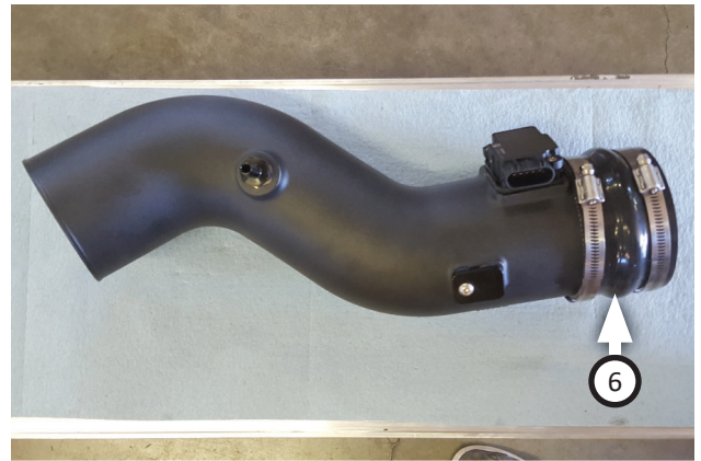
15. Place (x2) hose clamps (7) onto both sides of hump coupler (6) , then fit it onto MAF side of intake tube as shown.
