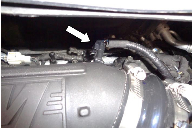
30. Push the MAF sensor plug onto the sensor until it clicks, then verify the connection is secure.
