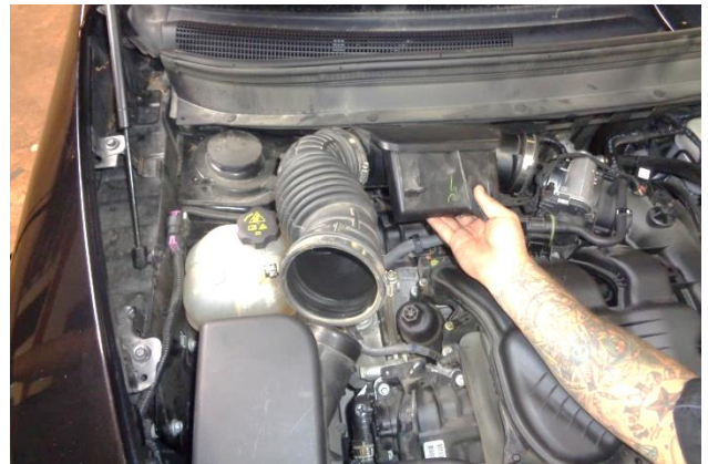
11. Separate the intake duct from the airbox and throttle body, and remove the duct from the vehicle.
