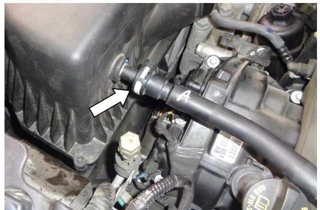
12. Disconnect the crankcase breather hose from the airbox.
