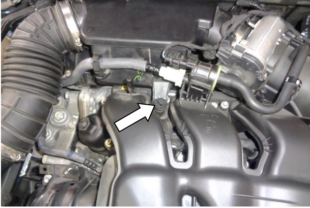
7. Release and remove the plastic push rivet at the front of the resonator.
