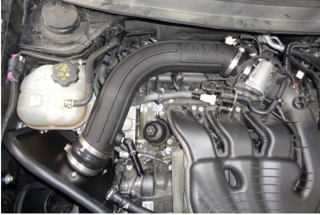
24. Install the intake tube between the heat shield and the throttle body.
