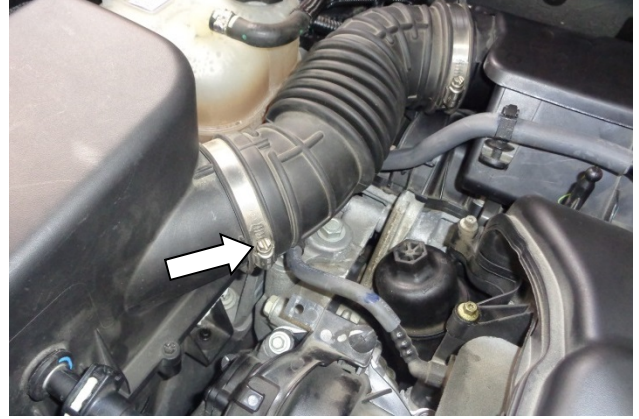
10. Loosen the screw clamp securing the intake duct to the airbox.
