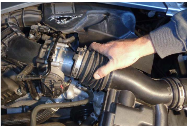
9. Loosen the hose clamp securing the intake duct to the throttle body, and remove the duct from the throttle body.
