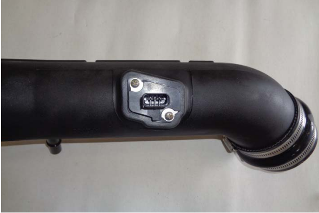
25. Slip the MAF sensor gasket (14) over the sensor, ensuring correct orientation. Then install the sensor in intake tube, using M4 screws (13).
