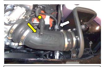
14. Insert the crankcase tube fitting ⇒ into the large grommet on the FM intake tube (the vent tube should be relaxed as shown ○) Next, reconnect the air-temperature sensor plug ⇒.
