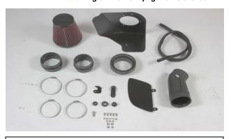
8. Begin the assembly process of the FM system by organizing the contents of the kit by thread and type. This will aid in the simplicity of this process and lessen the chance of misplaced parts.
