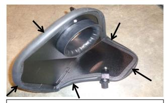
10. Install the air filter adapter using the 6mm screws and washers as shown. Install the rubber trim seal as shown by pressing fully into the groove starting from one end. Trim the final length with metal shears.
