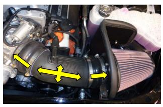
15. Install the FM air filter with the provided clamp. Adjust the FM intake tube endplay/rotation ⇔ to center between the fully seated rubber couplers ⇒. Align and tighten all hose clamps for a satisfactory fit.
