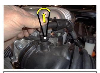
3. Disconnect the crank-case vent hose fitting from the stock intake tube by gently pulling straight up in an orbital motion. To make removal easier, spray a lubricant into the rubber connection point to act as a release agent for the fitting barbs.
