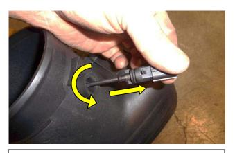
6. Remove the air temperature sensor from the factory air-box by gently lifting the clocking tab outward with a flat screwdriver and rotating counterclockwise as shown.
