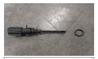
7. Remove the o-ring from the stock air temperature sensor and lubricate the o-ring area with a small amount of sensor-safe silicone grease or equivalent lubricant. Retain sensor for reinstallation later.
