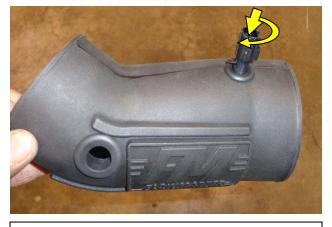
11. Assemble the FM intake tube as shown using the two provided rubber grommets. Install the stock air-temperature sensor into the small grommet as shown by pressing in and twisting clockwise.
