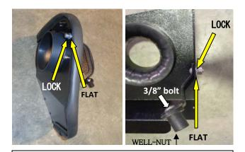
9. Loosely attach the two provided metal brackets to the heat shield using the ¼" cap screws/nuts and corresponding flat and lock washers → and the well-nut with corresponding 3/8" bolt → as shown.
