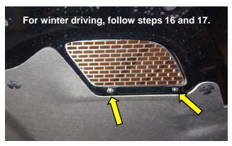
16. Install the provided drivers-side hood vent cover by removing the two fasteners ⇒ securing the stock hood screen. Keep the screen in place for reuse.
