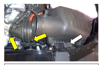
4. Loosen the hose clamps → which secure the factory intake tube to the throttle body and air-box. Detach from the air-box by compressing the intaketube bellows towards the engine. Remove the bolt → for the factory air-box on the front cross frame.
