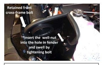
13. Combine the FM intake tube and the FM air-box assembly and install into the vehicle as shown. Tighten all fasteners including the well-nut\*. Leave the intake tube hose clamps loose for adjustment.
