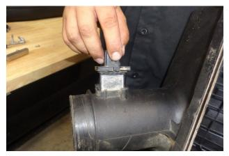
6. Remove the MAF sensor from the airbox cover, then remove the factory gasket from the sensor. CAUTION: The sensor is delicate! Handle it with care, and put it in a safe place until reinstallation.
