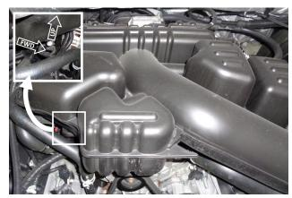
14. To release the duct-resonator from the throttle body, carefully work it side-to-side while pulling it forward. After it clears the throttle body, lift it upward to release its two mount pins from their grommets, and carefully remove it from the vehicle.
