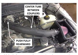
26. Push the rear coupler up against the stops on the throttle body, and tighten the throttle body clamp. Then center the intake tube between the couplers, and tighten the last two screw clamps.
