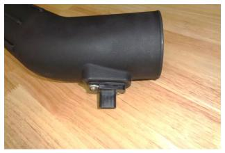
19. Slip the MAF sensor gasket (11) over the sensor, ensuring correct orientation. Then install the sensor in intake tube, using the M4 screws (12).
