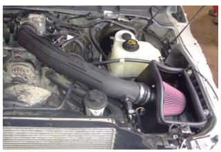
29. Secure the vacuum hose that was released from the resonator at Step 13, to prevent chafing or other damage to the hose or nearby components.
