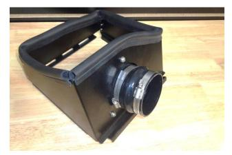
20. Slip the two smaller screw clamps (8) onto the 3-1/2" coupler (9). Install the coupler on the air filter adapter, pushing it flush against the heat shield. Tighten only the filter adapter clamp at this time. (Leave the other clamp loose.)
