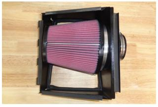
21. Slip screw clamp (2) onto air filter (1), then install the filter on the filter adapter and tighten the clamp.
