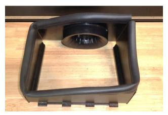
16. Firmly press the gasket (18) onto the edge of the heat shield, gradually working your way around. When you return to the starting point, use metal-cutting shears to trim the gasket to length.
