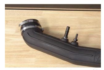
23. Slip the two larger screw clamps (16) onto the 3-3/4" coupler (17). Install the coupler on the other end of the intake tube. Only snug – do not tighten – the tube clamp at this time. (Leave the other clamp loose.)
