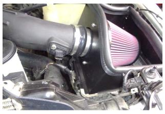
25. Secure the heat shield to the airbox with the three latches.
