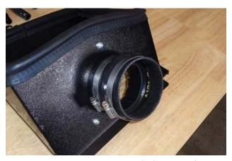
13. Slip the 2 larger screw clamps (10) onto the flex coupler (11). Install the large end of the coupler onto the air filter adapter, pushing it flush against the heat shield. Tighten only the filter adapter clamp at this time. (Leave the other clamp loose.)
