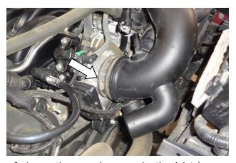
6. Loosen the screw clamp securing the air intake duct to the throttle body.
