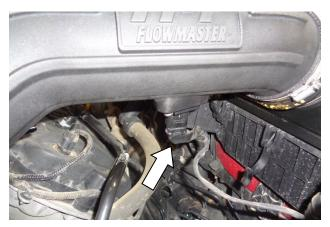
23. Reinstall the MAF sensor plug on the sensor, close the locking tab, and verify that the connection is secure.
