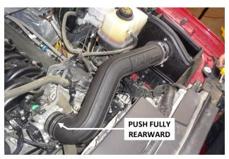
20. Push the straight coupling up against the throttle body and tighten the throttle body clamp. Then center the intake tube between the couplers (equal amounts of tube inserted in each coupler), and tighten the last two screw clamps.
