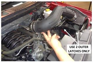
19. Insert the four tabs on the heat shield into the slots on the airbox. Lower the intake tube and install the straight coupling on the throttle body. Secure the heat shield to the airbox with the two outer latches. NOTE: The center latch is not used.
