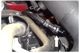
22. Connect the PCV hose to the quick-connect elbow, close the latch on the connector, and check the security of the connection.
