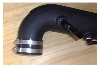
16. Slip the 2 smaller screw clamps (19) onto the straight coupler (20), then push the coupler onto the intake tube. Snug (do not tighten) only the tube clamp at this time. (Leave the other clamp loose.)
