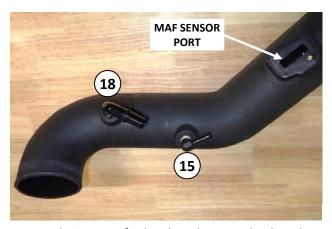
15. Apply 2 wraps of nylon thread tape to the threads of the 5/8" quick connect elbow (18) and the 3/8" barbed elbow (15). Install the elbows in the intake tube (14), oriented approximately as shown.
