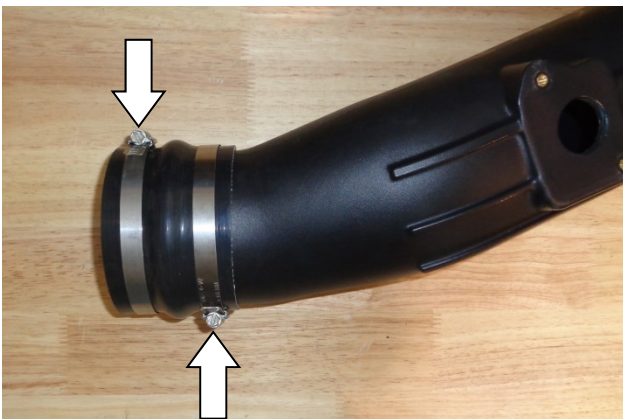
21. Install the two small screw clamps (23) on the flex coupler (24) with their screws oriented as shown , and install the coupler on the small end of the intake tube. Do not tighten the clamps at this time.
