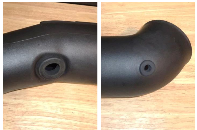
18. Insert the rubber grommets (22) and (19) in their holes in the intake tube (18). Moistening the grommets with soapy water will ease insertion.
