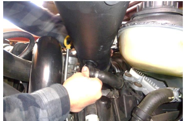
23. Lower the intake tube into alignment with the turbo inlet and carefully work the PCV tube into the grommet.
