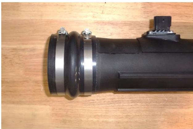
20. Slip the 2 large screw clamps (10) onto the flex coupler (9). Push the coupler onto the filter-end of intake tube. Snug the tube clamp (do not tighten at this time), and leave the other clamp loose.
