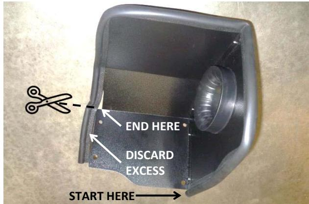
15. Attach the gasket (4) to the heat shield. Starting at the bottom of the front edge, firmly press the seal onto the edge, gradually working your way around. At the bottom of the opposite edge, trim the seal using metal-cutting shears.
