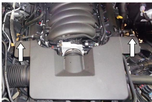
6. Locate the two PCV hose connectors at the back of the intake plenum as shown.
