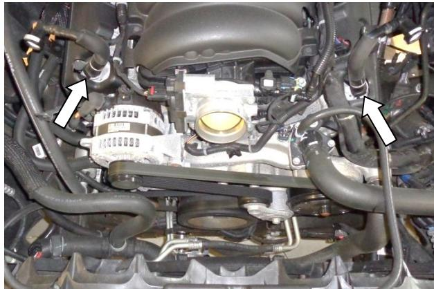
10. Remove both PCV hoses from the valve covers by depressing their release latches and pulling straight off.
