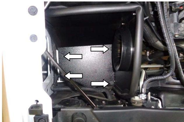
16. Use the 4 bolts retained at Step 12 to install the assembled heat shield in the vehicle. **NOTE: At each location, be sure to use the same length bolt as was removed (see Step 12).**
