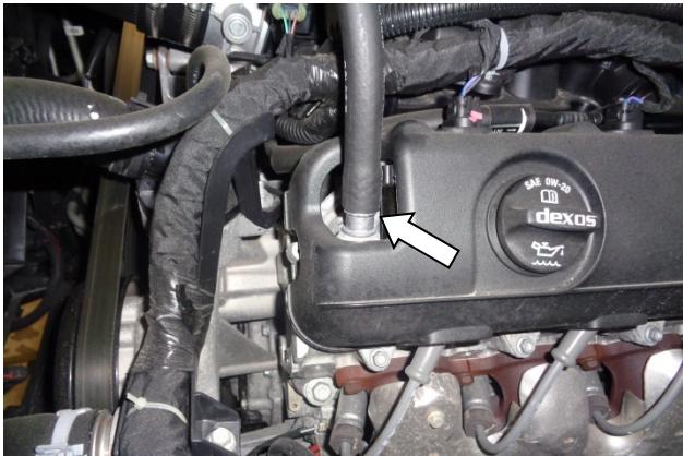
24. Install a hose on the PCV port on each valve cover (2 places). Push each hose fully onto the port, until it touches the raised lip.
