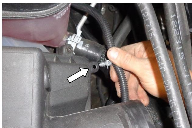
5. Release the clamp holding the MAF sensor wire from the corner of the airbox.
