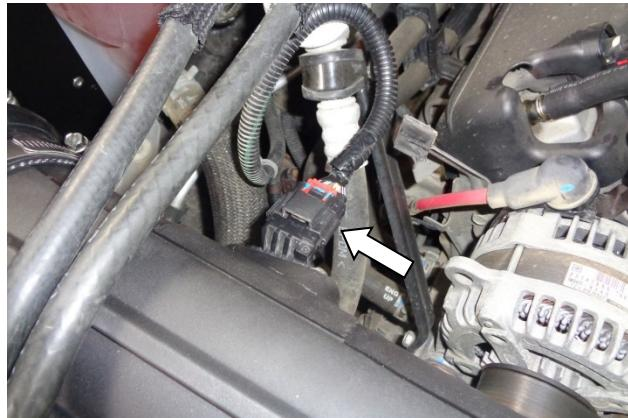
26. Reconnect the MAF sensor plug to the sensor, close the locking tab, and verify that the connection is secure.
