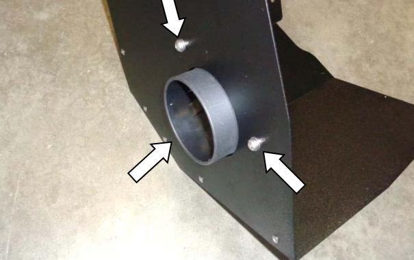
14. Assemble the air filter adapter (3) to the heat shield (5) using the M6 screws (8), lock washers (7) and flat washers (6).
