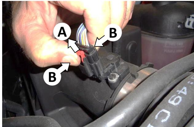
4. Disconnect the mass airflow (MAF) sensor plug by:
