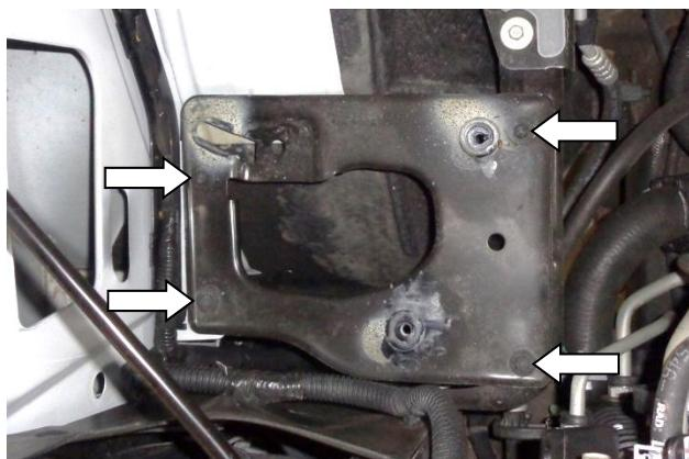
12. Remove the airbox shelf by removing its 4 mount bolts. Retain the bolts for reinstallation at Step 16.
