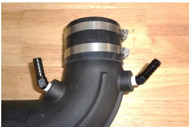
19. Slip the 2 small screw clamps (17) onto the straight coupler (18). Push the coupler onto the throttle body-end of the intake tube. Snug the tube clamp (do not tighten at this time), and leave the other clamp loose.
