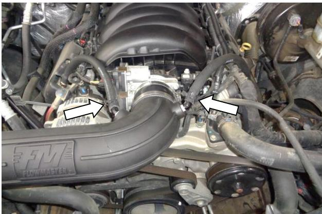
25. Push the other ends of the hoses onto the barbed elbows and secure with pinch clamps (15).
