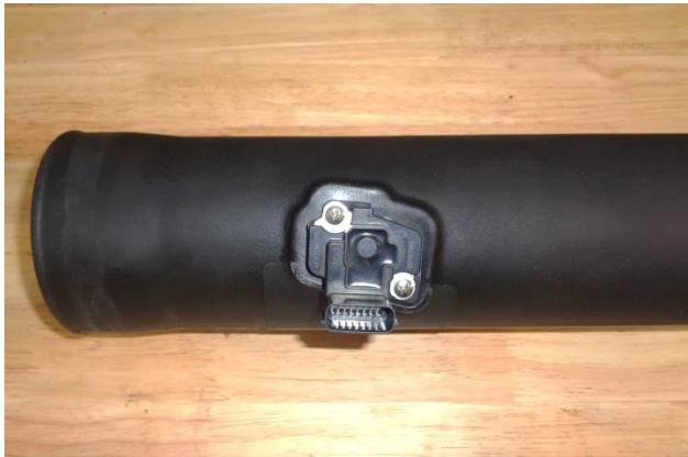
18. Install the MAF sensor gasket (11) onto the sensor, ensuring correct orientation. Then install the sensor in the intake tube, using the M4 screws (12).
