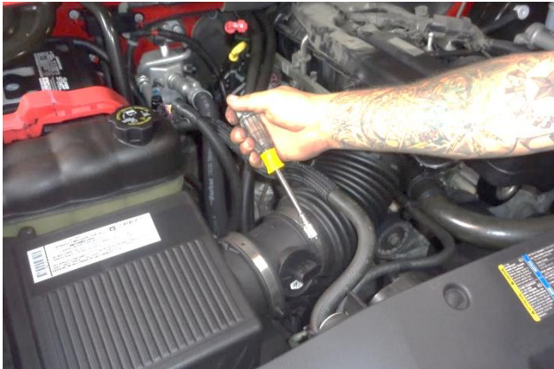
8. Loosen the hose clamp securing the air intake duct to the MAF sensor, then disconnect the intake duct from the MAF sensor.
