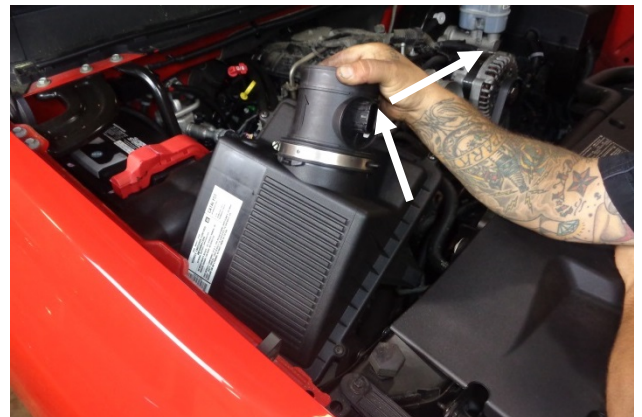
12. Remove the assembled airbox and MAF sensor by grasping the sensor and lifting straight up (to release the airbox mount pins from their rubber grommets), then sliding the airbox inboard to release it from its shelf.
