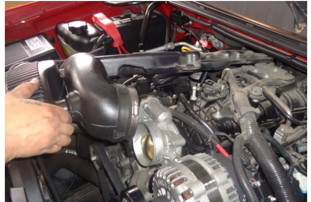
11. Disconnect the intake duct from the throttle body, and remove the duct from the vehicle.
