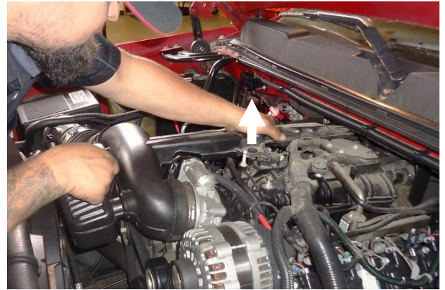
10. Lift the intake duct resonating chamber straight up, just enough to release it from its friction clip.
