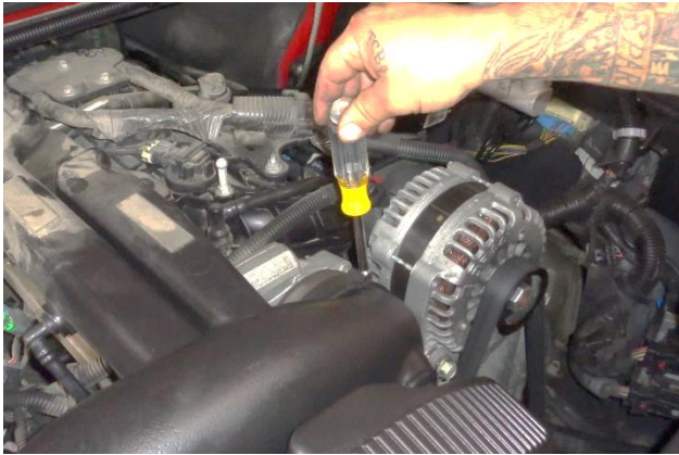
7. Loosen the hose clamp securing the air intake duct to the throttle body..
