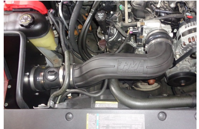
27. Adjust the intake tube as necessary to avoid contact with surrounding components (such as the radiator hoses). When the tube is aligned as desired, tighten the two tube clamps.
