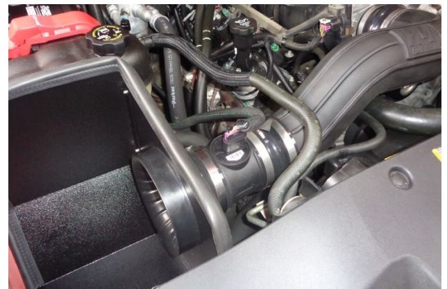
29. Plug the MAF sensor lead into the sensor until it clicks, then verify the connection is secure.
