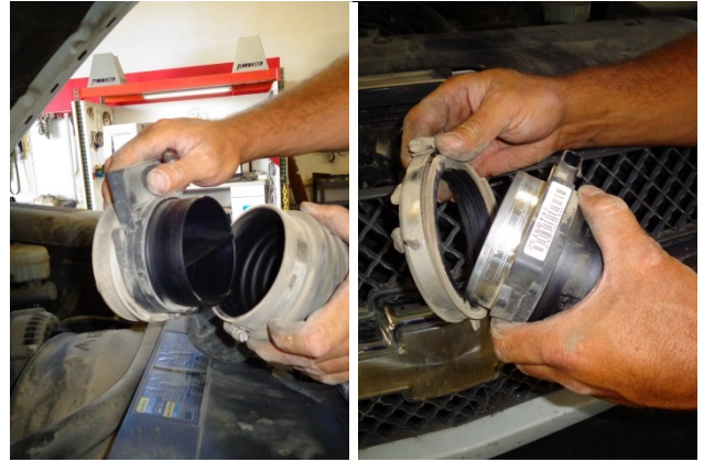
10. Loosen the screw clamp securing the MAF sensor to the intake duct and remove the sensor. Remove the clamp and rubber seal from the sensor. CAUTION: The sensor is delicate! Handle it with care, and place it in a safe location until reinstallation.
