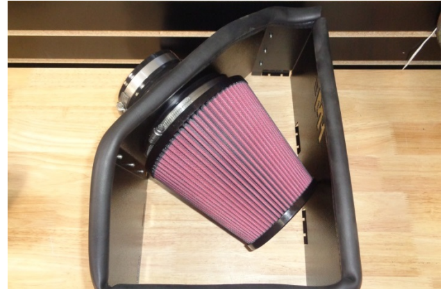
16. Place the clamp (2) on the air filter (1), install the filter on the filter adapter and tighten the clamp.
