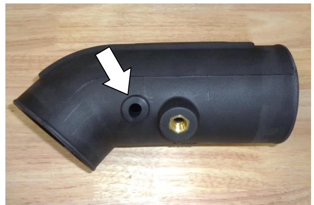
18. Insert the rubber grommet (14) into the intake tube (16). NOTE: Moistening the grommet with soapy water will ease insertion.
