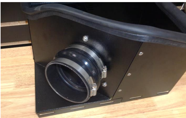
15. Slip two of the large screw clamps (10) onto the flex coupler (9). Install the coupler on the air filter adapter, pushing it flush against the heat shield. Tighten only the filter adapter clamp at this time. (Leave the other clamp loose.)
