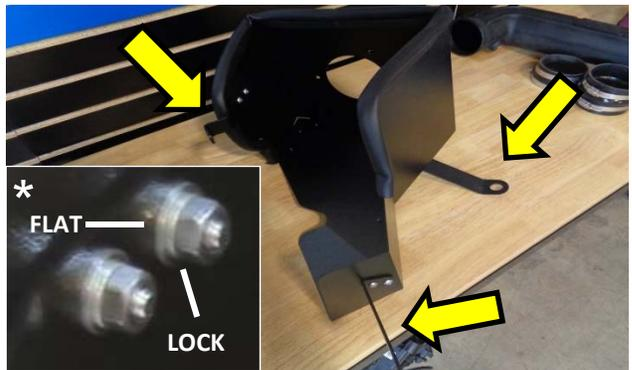
10. First, attach the 3 metal brackets → to the FM heat-shield using the supplied ¼" bolts/nuts and corresponding flat/lock washers installed under the nut-side as shown\*. Tighten all fasteners securely.
