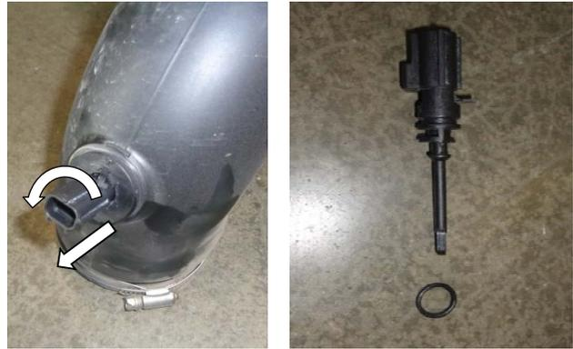
4. With the stock air intake assembly lying on a flat surface, remove the stock air temperature sensor from the intake tube by twisting counter-clockwise and gently pulling outward simultaneously. Next, remove the O-ring from the sensor body and lube the area with a sensor-safe grease. Retain in a safe place.
