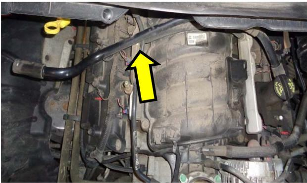
7. Remove the crankcase vent tube → from the engine. Replace the stock tube with the included hose/clamps. Route in the same path, trimming off any excess length after install of the FM system.
