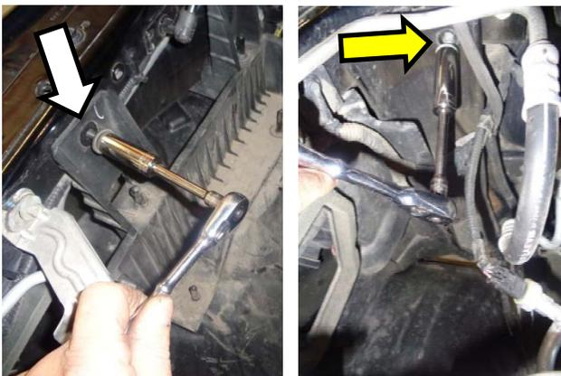
8. Remove the front retaining bolt → from the stock air-box frame on the fender and retain. Next, remove the bolt on the front cross-frame behind the headlight assembly as shown → and retain.
