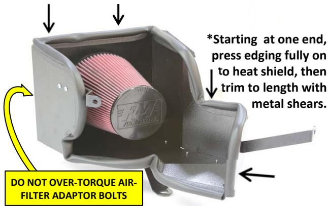
12. Using the (3) three 6mm bolts/washers, secure the air-filter adaptor to the heat-shield assembly. Next, install the rubber edging as above \*, then securely attach the provided FM air-filter/clamp assembly.
