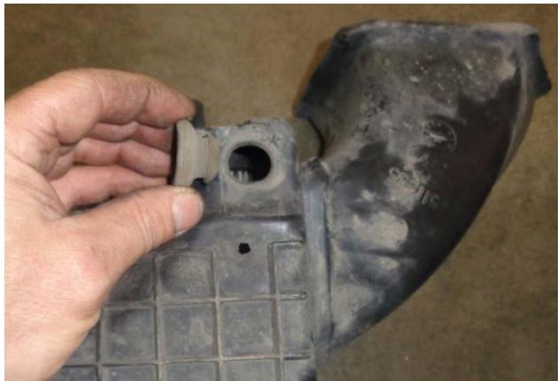
5. Turn the stock air intake assembly over and remove one of the rubber grommets from the base and retain for use on the FM Cold Air Intake System.
