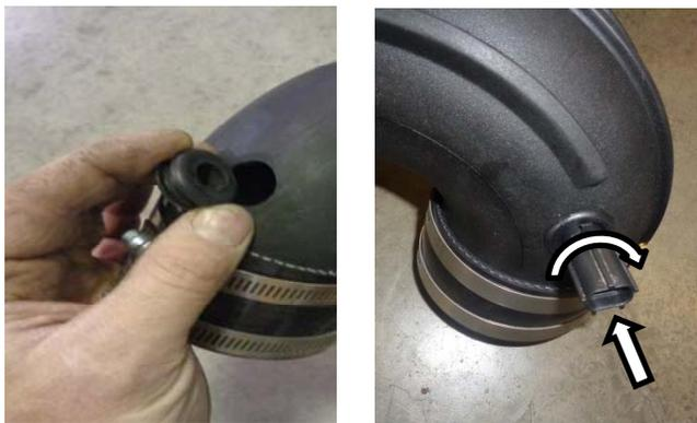
14. Install the provided rubber grommet into the hole on the FM intake tube and insert the previously retained air temperature sensor fully by twisting clockwise and pressing in at the same time.
