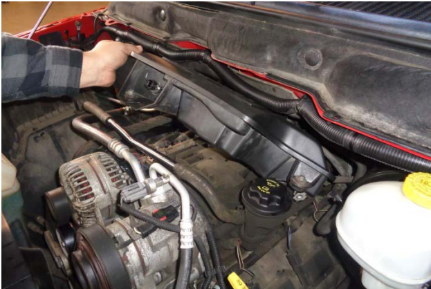
8. Remove the resonator from the vehicle.
