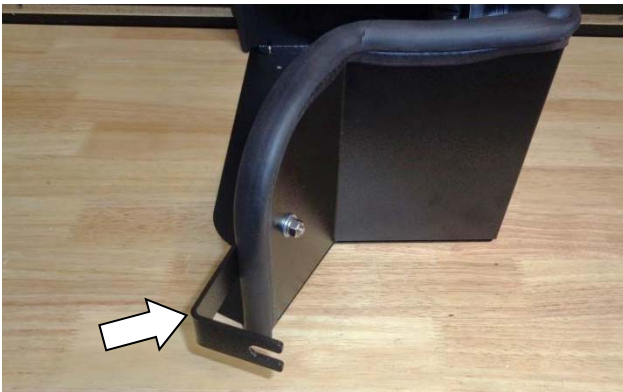
15. Attach bracket (11) to the heat shield using a ¼-20 screw (8) (on the bracket side), and flat washer (4), lock washer (5) and nut (6) (on the heat shield side). Do not fully tighten the fasteners at this time.
