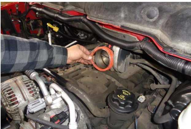
9. Remove the rubber gasket from the throttle body.
