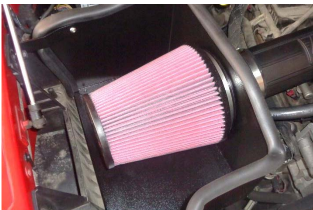
28. Place clamp (2) on air filter (1), install the filter on the filter adapter, and tighten the clamp.
