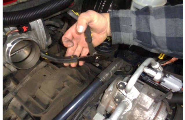
10. Disconnect the PCV hose from the base of the oil filler neck and remove the tube from the vehicle.
