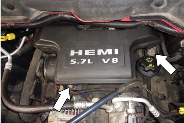
7. Loosen the two resonator bolts. (Bolts are captured / not removable.)
