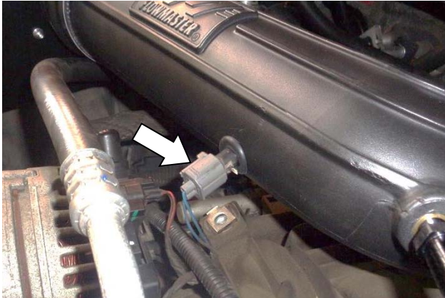
31. Connect the air temp sensor plug to the sensor and check the plug for security.
