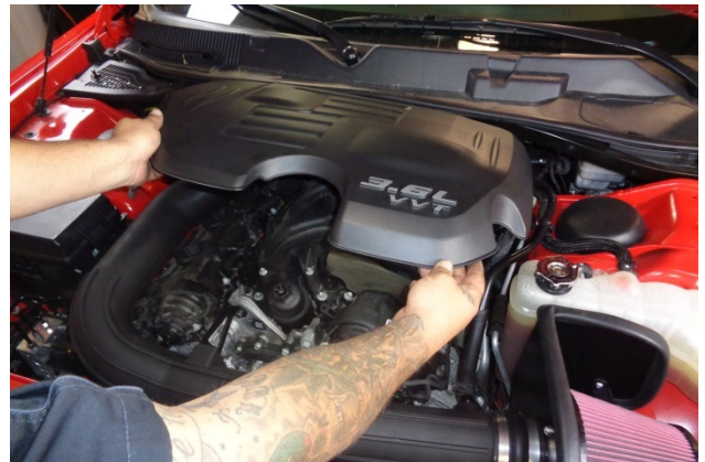
29. Align the engine cover over its four mount posts, then snap it into place at all four corners.
