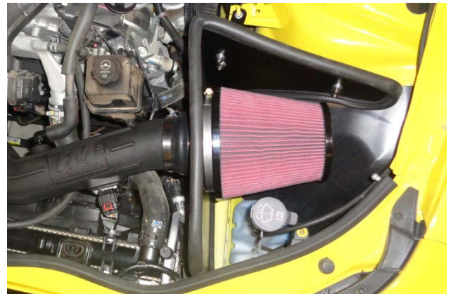
23. Install clamp (2) on air filter (1), install filter on filter adapter and tighten clamp.
