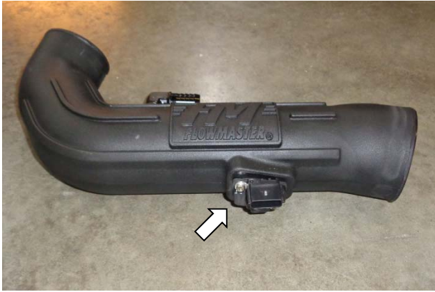
18. Install MAF sensor gasket (21) onto the sensor, ensuring correct orientation. Then install sensor in intake tube, using M4 screws (22).
