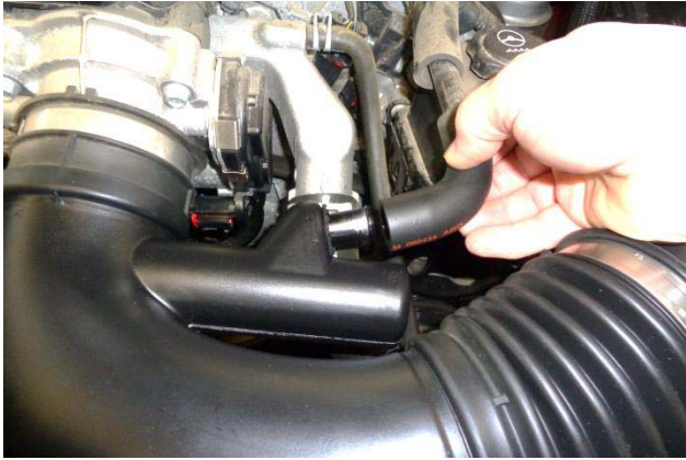
7. Disconnect the positive crankcase ventilation (PCV) tube from its fitting on the intake tube.
