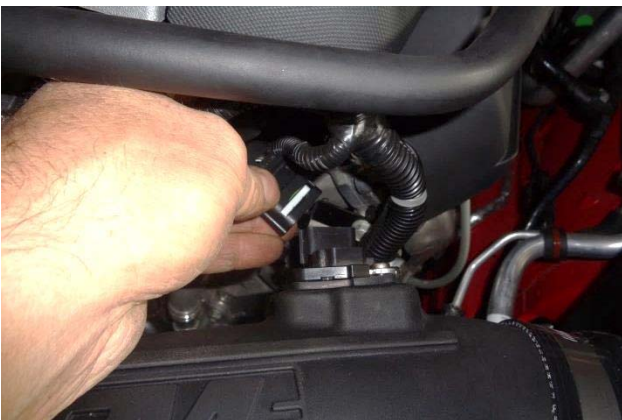
26. Install MAF sensor connector and check for security.
