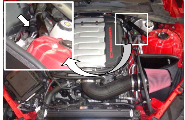
28. Install dust cap (17) on open end of resonator hose.
