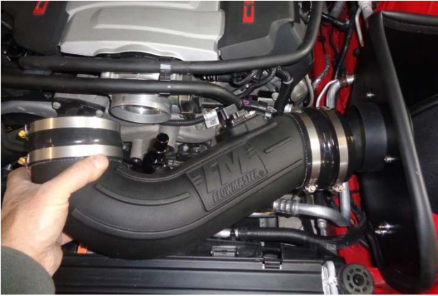
24. Install assembled intake tube in vehicle and tighten all hose clamps.
