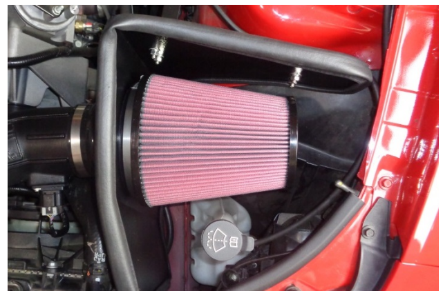
24. Place the clamp (2) on the air filter (1), install the filter on the filter adapter and tighten the clamp.
