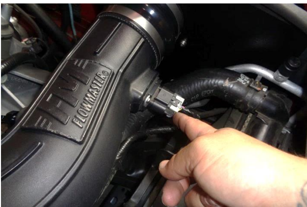
21. Install the MAF sensor plug on the sensor, and push the locking tab toward the sensor. Then check the plug for security.
