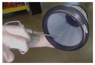
3. <u>Blow through</u> the filter, from the inside out. Keep the nozzle moving; do not hold it stationary over one place on the filter.
