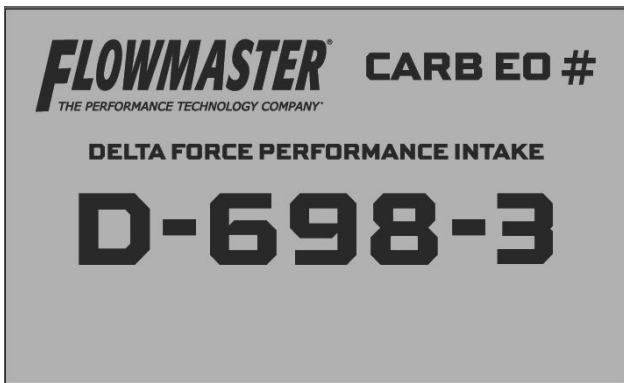
26. Affix the CARB Exemption Order label to a clean, readily-visible location under the hood (e.g., near the hood latch), so an inspector can easily see it at emissions testing.
