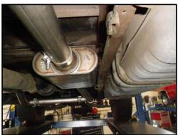
5) Place a supplied 2.50" clamp over the outlet of one of the **942545K** mufflers and slide onto the front of the right tailpipe, support the muffler with a stand and tighten the clamp enough to hold but still allow for adjustment. Repeat this step on the left side of the vehicle. Place another supplied 2.50" over the inlet of both mufflers.
