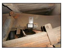
2) Locate the cross member at the front of the rear leaf spring, on the left side of this cross member, there will be a factory hole  $9.00^{\circ}$  in from the frame and  $3/4^{\circ}$  up from the bottom, this hole location will need to be duplicated on the right side of the vehicle. Measure over  $9.00^{\circ}$  from the frame and  $3/4^{\circ}$  up as shown in the photos below, use a center punch to make a mark and drill a  $5/16^{\circ}$  hole on this mark.
