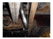
4) Take the **86076** muffler inlet pipes and place a supplied 2½" clamp onto the expanded end, place them onto the back of the H-pipe assembly's **86074** & **86075**. Rotate them up into their approximate position and tighten the clamps enough to hold but still allow for adjustment.
