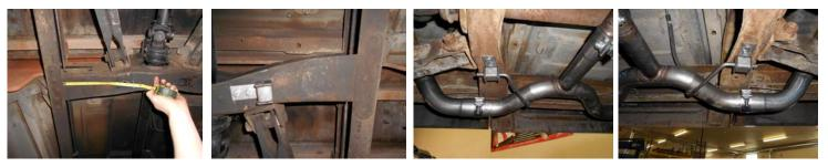
2) Take the right and left H-pipe assemblies, **86074** & **86075** and connect them together at the center cross-over connection. Place them up into position and connect the hangers on the pipe to the rubber mounts installed above. The hanger rods should stick thru the rubber block on the **HA572** hanger approx. 1.00". Support the front of the assembly with a stand. Place the provided 2" clamp at the center H-pipe connection.
