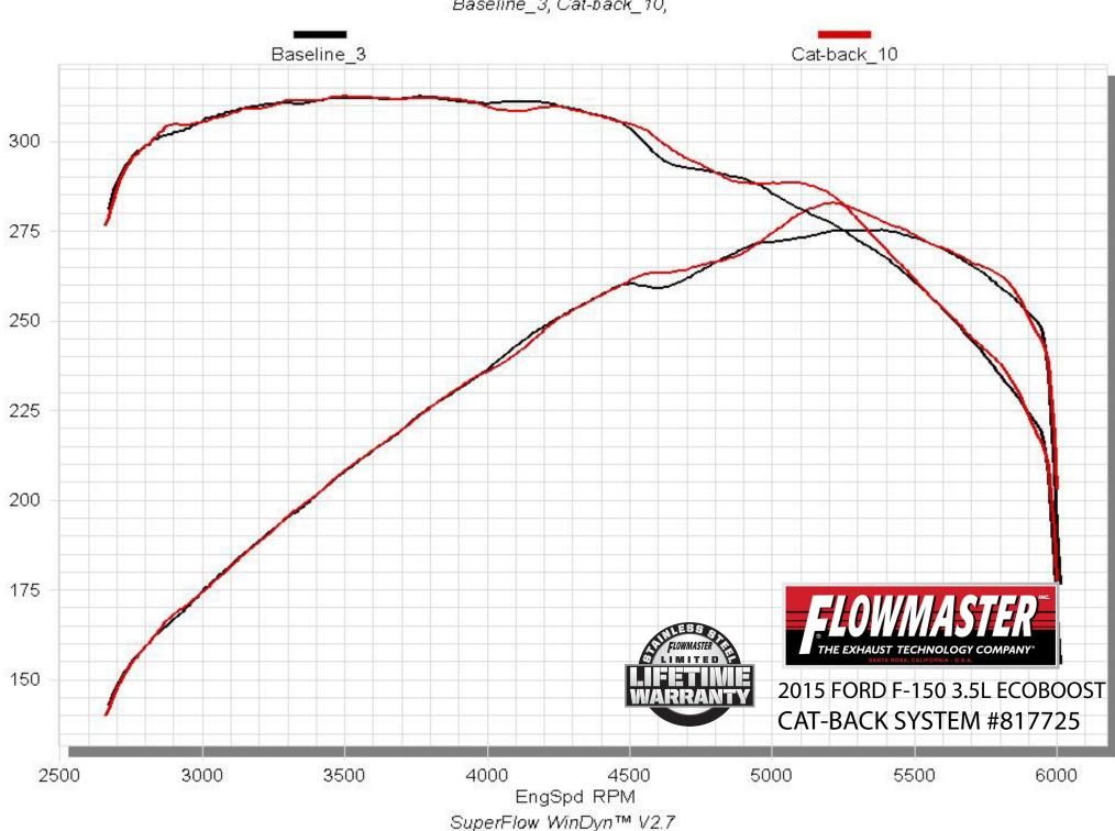
STP Corrected Wheel Power vs. RPM
