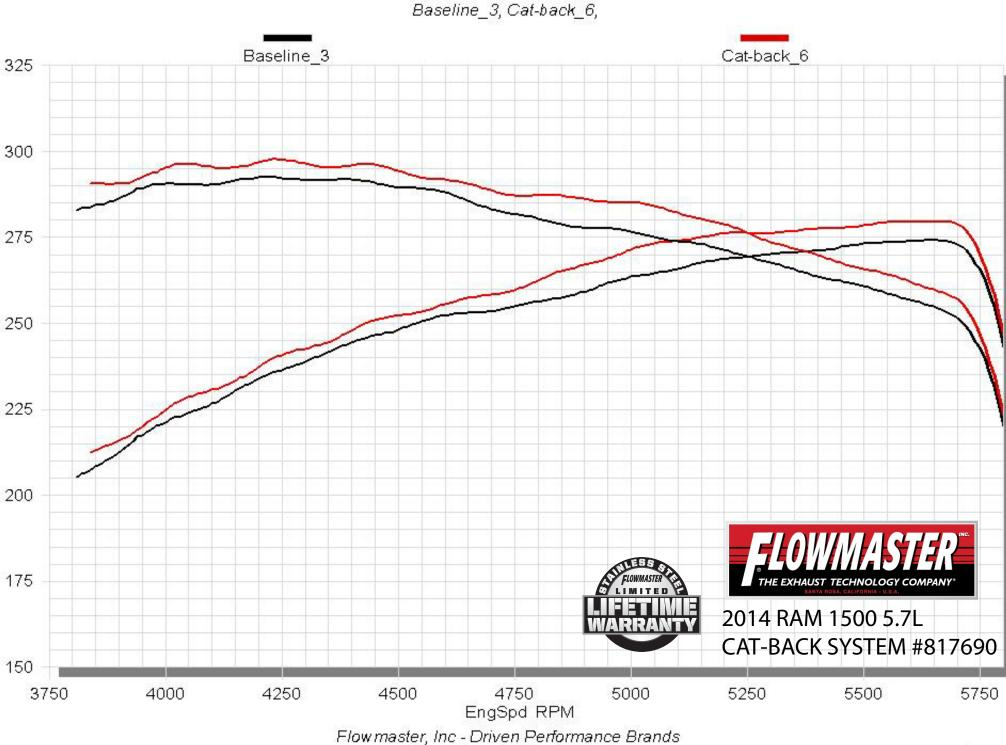
STP Corrected Wheel Power vs. RPM
