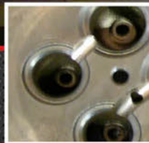
GRIND OUT CRACKS
