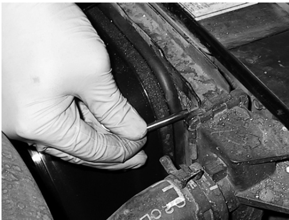
Install temp. probe near inlet hose...
