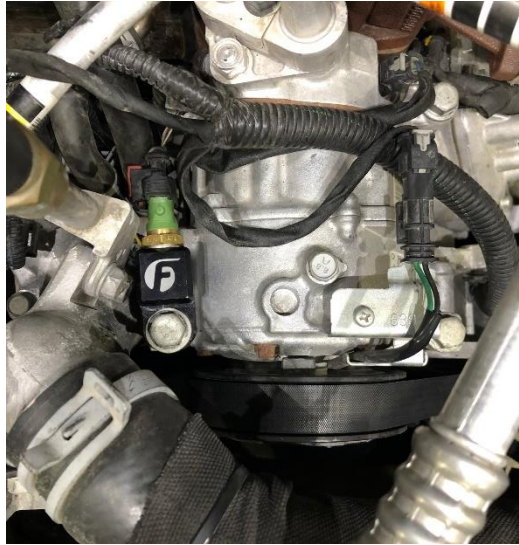
Fig. 17: Fuel temperature sensor block location
