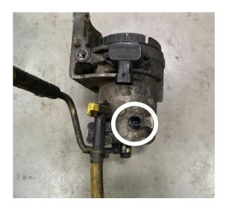
10. Install the WIF sensor in the bottom of the fuel filter delete or the supplied WIF sensor plug.
