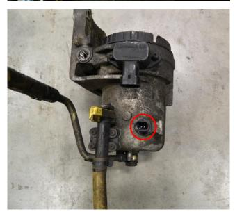
STEP 10: Install the WIF sensor in the bottom of the fuel distribution block or the supplied WIF sensor plug.
