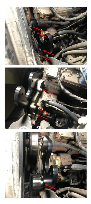
STEP 14: Install the high flow CP3 inlet fitting into the pump (item 1) as well as the M12 to -6AN fitting for the return.
