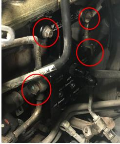
STEP 11: Install a M12 to -8AN fitting into the OEM low pressure feed of the factory CP3, route it using the two (2) -8AN 90 degree fittings to the bottom front feed fitting on the distribution block as shown.
