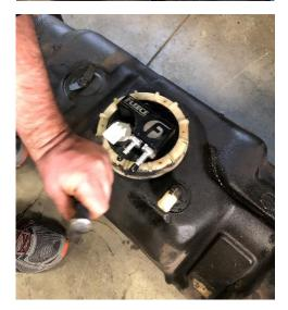
STEP 14: Transfer the fuel line locking tabs to the fuel lines or transfer them to the PowerFlo lift pump fuel line connections. A replacement locking tab is included in your kit.
