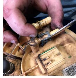
STEP 9: Remove the gasket from the tank.
