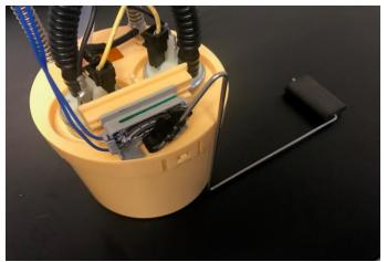
STEP 15: Install the PowerFlo pump assembly into the tank and reinstall the retaining ring using your hammer and punch or chisel by rotating it clockwise to the fully engaged position. Ensure proper orientation of the pump and fittings matches the orientation of the original pump.
