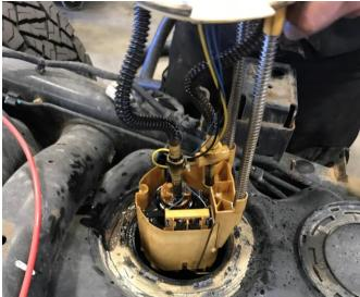
STEP 10: Clean the tank sealing surface and place your <u>new</u> o-ring supplied in the kit for the PowerFlo lift pump onto the top of the tank.
