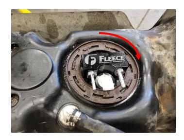
STEP 16: Make the proper connections for the fuel lines, vent, fill tube, and electrical connection. Make sure the quick disconnect fuel lines are fully seated with retaining clips in place. When the quick disconnect fitting is fully seated you will not be able to pull it back off the pump fitting without releasing the retaining clip.
