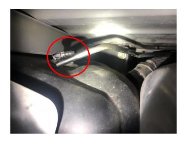
STEP 8: Remove the filler neck hose at the tank with a 9/32" socket to loosen the clamp. Access the clamp through the fender well.
