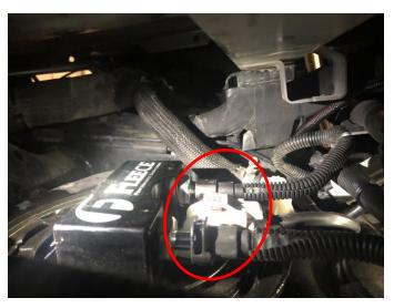
STEP 14: Connect the supplied electrical wiring harness to the OEM harness and PowerFlo lift pump.
