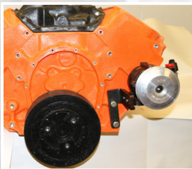
Install pump to bracket (2) using bolts (9) and washers (10) supplied
