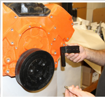
Install L-shaped bracket (2) on engine with bolts (16) and lockwashers (14) supplied
