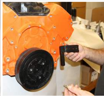
Install L-shaped bracket (1) on engine with bolts (15) and lockwashers (11) supplied
