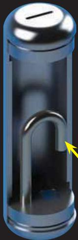
Cane-style baffle design in Reservoir prevents foaming in fluid
