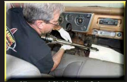
**Alignment Slot in New Column**
