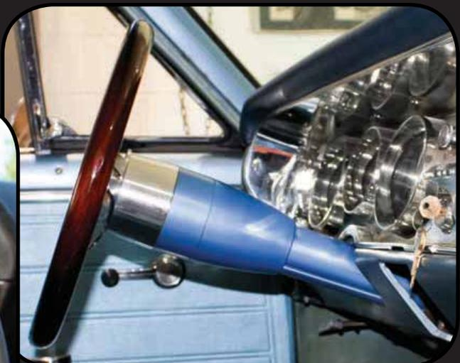
**FR20143** 67 & Prior Wheel Adapter installed on a 66 Chevelle Steering Column.
