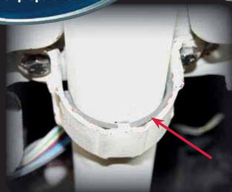
Place included rubber spacer into the factory under dash mount and trim away excess.
