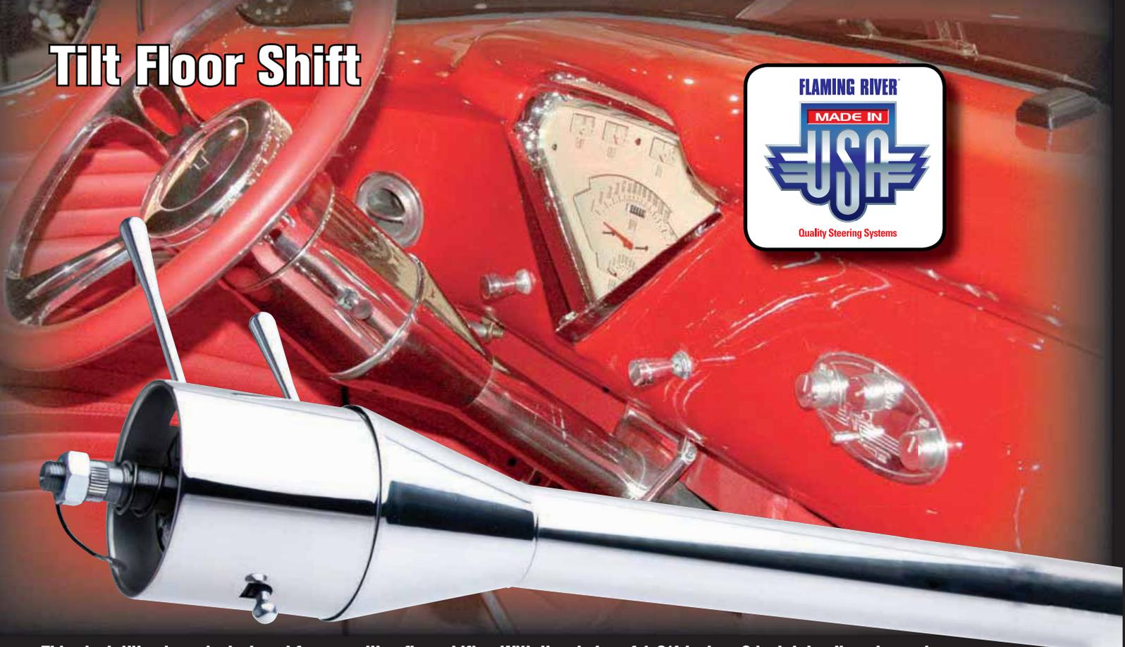
This sleek tilt column is designed for use with a floor shifter. With the choice of 1-3/4 inch or 2 inch tube diameter and a compact shroud, you create a unique, new custom look. Each column comes complete with a billet aluminum dress up kit, GM turn signal with hazards, a 4-1/4 inch connector and canceling cam. Standard shaft size is 1 inch DD and you can choose from paintable, polished or black powder coat.
