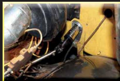
**U-Joint and Shaft Installation**
