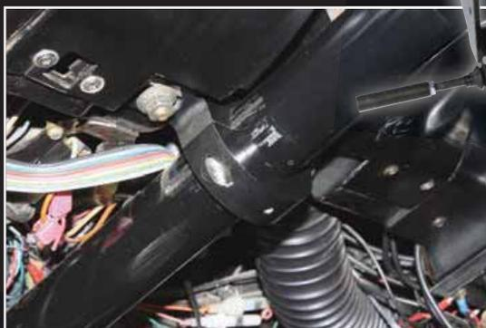
Install the upper portion of the new Flaming River® Mounting Clamp into the stock location.
