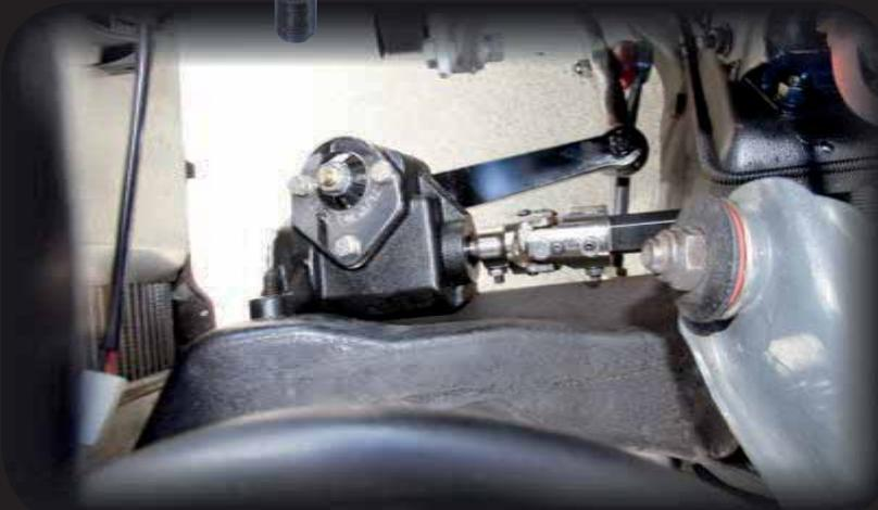
Vega Steering Box installed in a 1976 Nova
