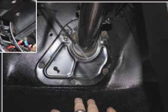
Slide the new steering column through the opening in the original floor mount, and then slide the column through the opening in the firewall.
