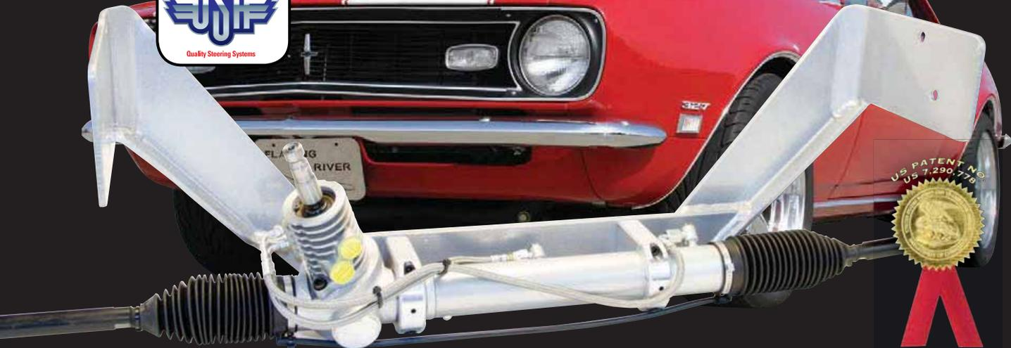
Flaming River has designed a direct bolt-in steering system that utilizes a power rack and pinion engineered for your Classic Camaro! Like the manual kit, the power rack and pinion provides a quick steering ratio with full turning radius! The power rack and pinion installs easily (within hours) using the existing chassis hole locations. Available with or without steering column.
