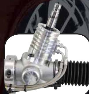
Rack and Pinion Valve reversed allows the pressure and return ports to face the backside of the rack.
