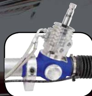
Rack and Pinion Valve in the standard position with the pressure and return ports facing forward.
