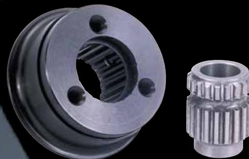
Features a precision-tolerance design for positive steering input. Uses a standard 3-bolt mounting pattern and can be used with Flaming River FR20119 Billet Aluminum Wheel Adapter to fit 5 and 6-bolt steering wheels. 20-spline design fits 3/4" smooth shaft and utilizes deep beveled splines for a greater engaged surface area. Meets SFI-Spec 42.1 requirements with a NASCAR-required steel pull disconnect ring.
