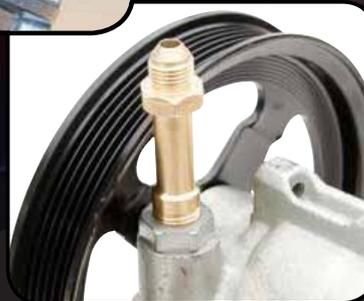
**LS3 Power Steering Pump Extended AN Fitting**
