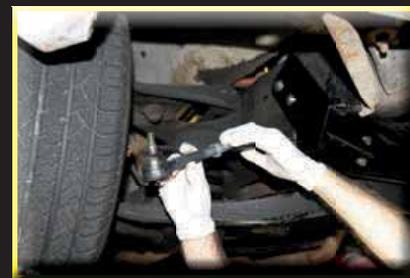
**Install The Outer Tie Rod End**
