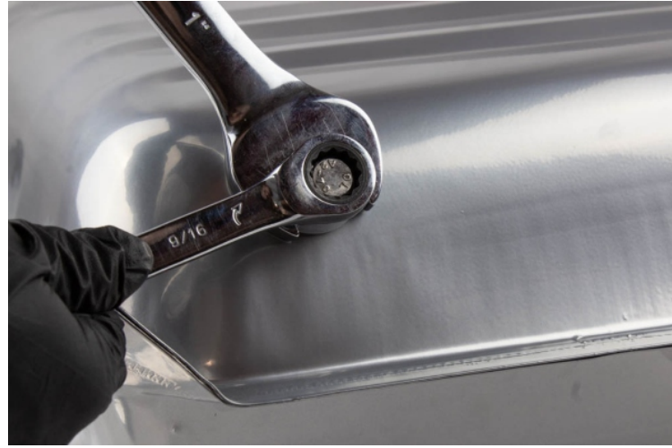
Twist bolt to collapse and set bung.
