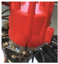
4- Line up the center of the reluctor wheel (this is the 8 paddle wheel) with the center of the pickup on the distributor. See the photo at bottom of page. Use a light to make sure you are centered and snug down the
