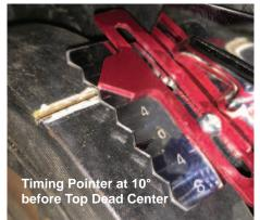
evant for this setup example. Drop your distributor in place like you normally would with the rotor pointing at the #1 spark plugposition. 2- On the keypad you will input this number under Ignition Setup Distributor Base Timing This can be done later during the setup mode. We are just showing you where you will be entering this number and where it comes into play.
