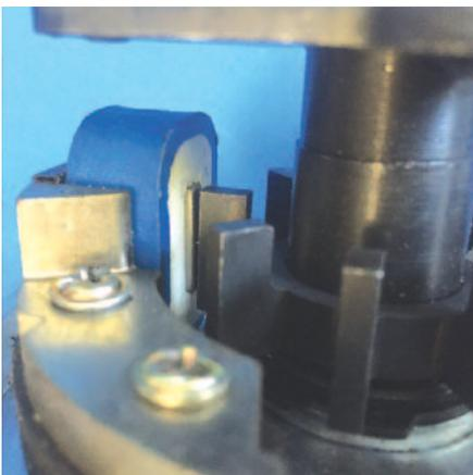
ECU. Make sure the rotor is in the center position and that it is pointed at the mark you made for the #1 spark plug location. Remove the rotor if it helps you see the re-lector position better.
