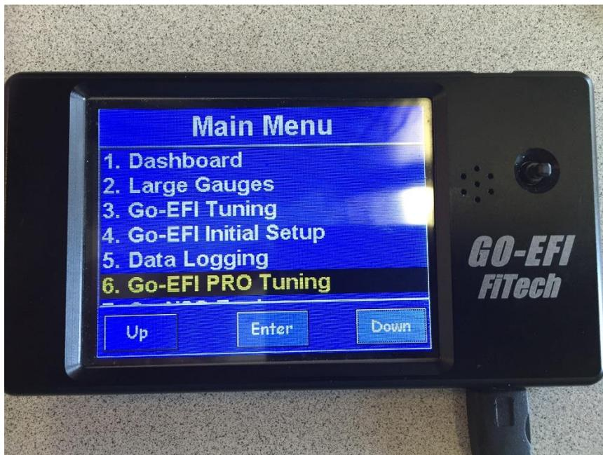
Step 3: In the Go EFI Pro Tuning Menu scroll down to Option 12 Fuel Pump Control. Select Fuel Pump Control.
