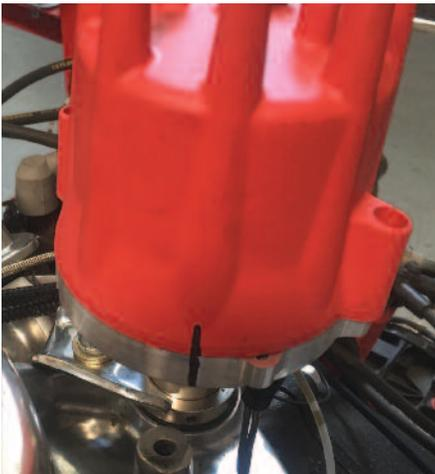
4- Line up the center of the re-lector wheel (this is the 8 paddle wheel) with the center of the pickup on the distributor. See the photo at bottom of page. Use a light to make sure you are centered and snug down the distributor. You may need to move the distributor slightly later to get final synchronization with the
