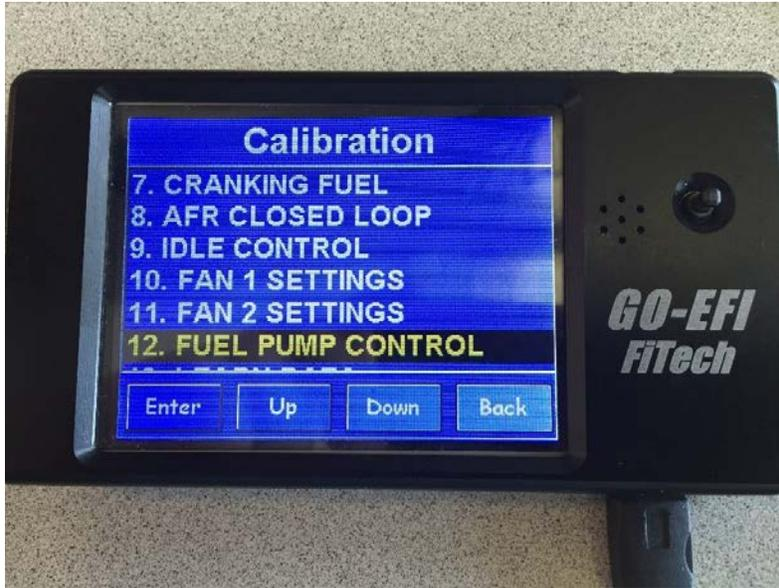
Step 4: Scroll down to option 7 (PWM Low Flow) select edit. In the edit menu press clear (CLR) enter a new value of 40.
