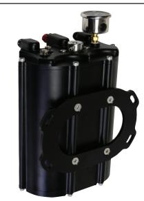
The heavy duty bracket can be installed on the bottom (shown above) or side of the tank to ease mounting. The all new Force Fuel System makes the upgrade to FiTech EFI even easier! The Force Fuel System mounts under the hood and is fed with the original mechanical or electric fuel pump then supplies the EFI system with the required high pressure through the use of an internal 340-LPH pump. This means you don't need to run a new feed line from the tank!
