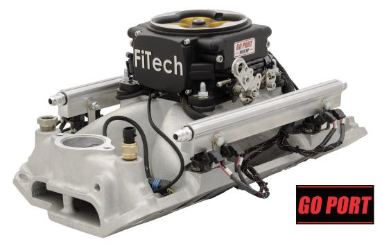
The Go Port EFI system features eight injectors placed precisely in each intake runner to inject fuel right into the cylinder head port. A sequential port fuel design provides excellent throttle response, effective fuel atomization and delivery resulting in terrific throttle response and overall performance.
