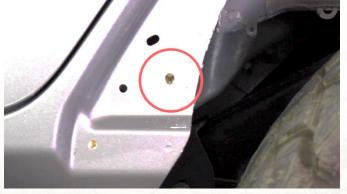
With a 7/16" drill bit, drill out the hole.
