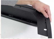
Lift your <u>new fender flares</u> into place. Line up the holes in the fender flare with the Jeep's OEM holes. Attach the flare with the supplied bolts, washers and nuts.
