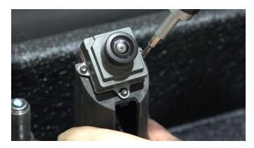
Using a T-6 Torx bit unscrew the Backup camera from its mount. And remove the camera feed cable. Carefully place the camera aside.
