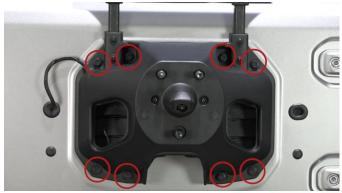
Using a 13mm Socket remove the eight tire carrier bolts. Using a T-25 Torx bit remove the backup camera retaining plate, pull the camera free from the backside of the tire carrier.
