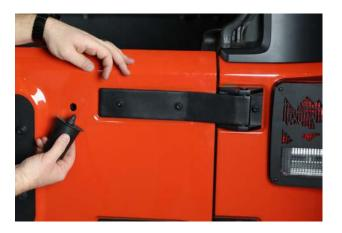
Insert the two smaller grommets into the rubber stopper holes.
