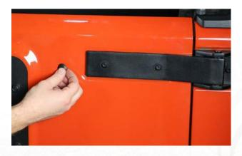
Insert the larger grommet into the larger hole the OEM brake light harness ran through.
