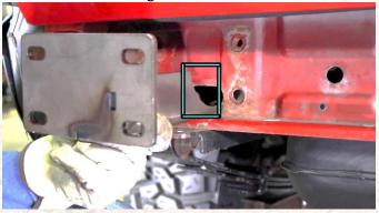
Trace the brace's rail dimensions onto the body, giving you a line to follow while cutting.
