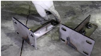
Hold the brace's rail up to the frame rail, inbetween the mounting bolt holes.
