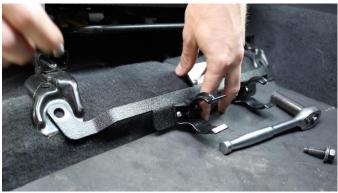
The seat safety rated torque specifications for each bolt is 27ft-lbs.
