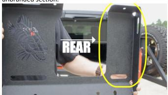
As shown above, this section will always face the rear of the vehicle, and the tub rail holes will cover your vehicle's (2) most rear rail holes.
