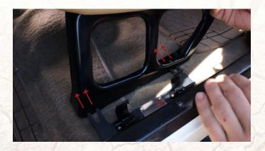
Secure it by tightening the seat bolts with a torque of 35 ft-lbs.
