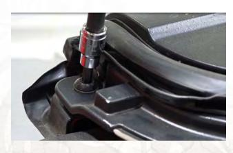
Remove the remaining six (6) torx bolts (3 on each side) from either side of the hard top from inside the Jeep.
